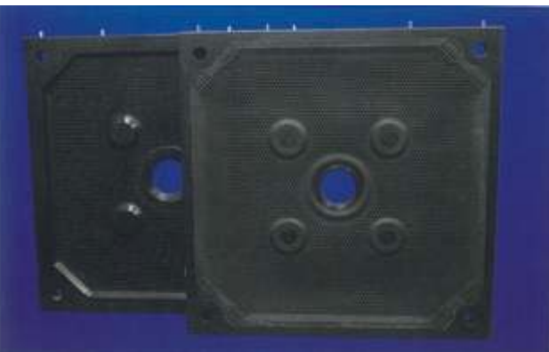
Membrane- and combination chamber plate 1200 x 1200 mm. PVDF plate and EPDM membrane are electric dischargeable. Application at extremely high temperatures and / or with aggressive chemicals.
