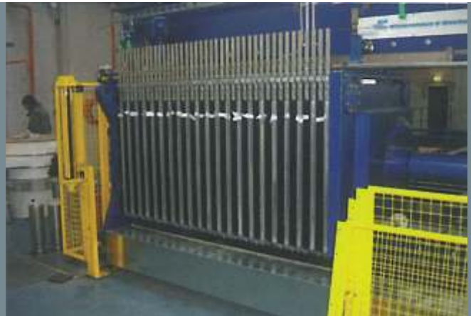
Filter press with membrane- and combination chamber plates 1200 x 1200 mm. Filtration of metal pigments with solvents, 16 bar squeezing pressure.
