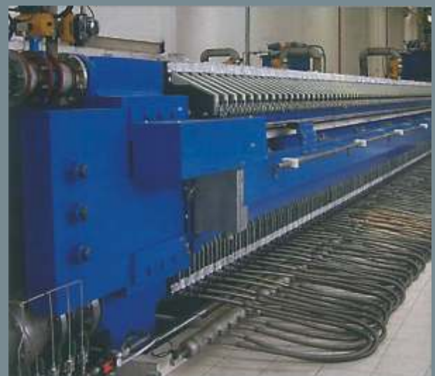
Filter press with high performance membrane chamber plates 1500 x 1500 mm up to 5,0 MPa (50 bar)
