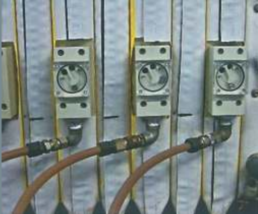
Squeeze Indicator Indication of the end of squeezing process. Early detection of leakages in the package. Installation in existing membrane chamber plates possible.
