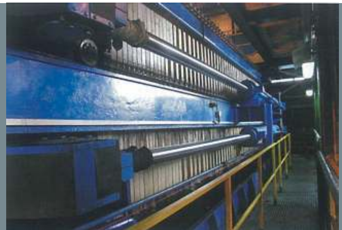
SALA filter press with JVK membrane- and combination chamber plates 1500 x 1500 mm
