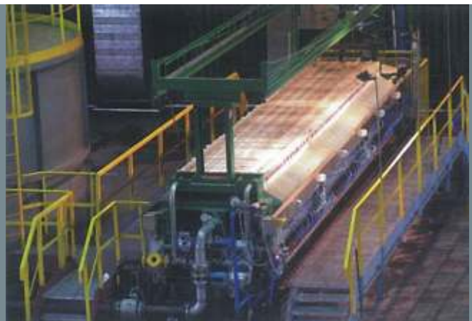
Filter press with PVDF membrane- and combination chamber plate 1200 x 1200 mm, application metallurgy, chemistry etc.
